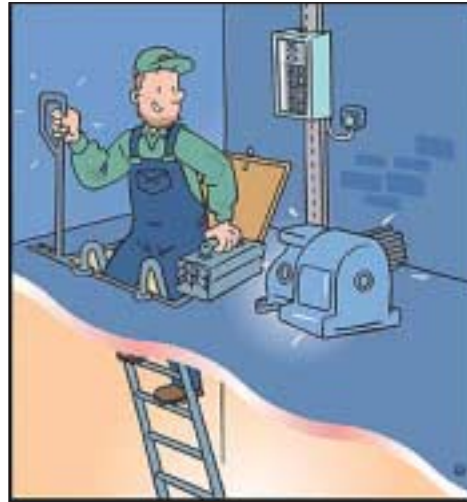
Install the necessary ladder, handrail & equipment for a safe and easy access to the machine room
