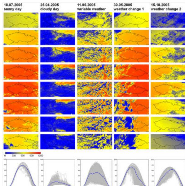
**Figure 6:** Maps showing variability of solar radiation in the Czech Republic, and graphs of the respective daily profiles of PV power generation at the level of ČEPS Transmission System (blue line) and also daily profiles of randomly selected 1 MWp PV power plants.
