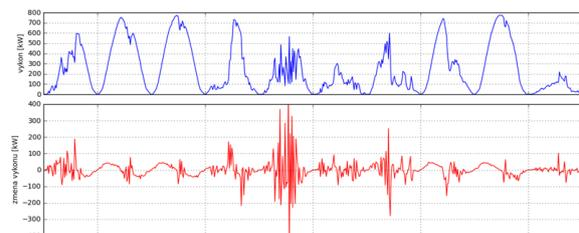
**Figure 4:** Generation profile of a single 1 MWp PV power plant (blue) and the corresponding absolute variability (red), assuming 15-minute time step.
