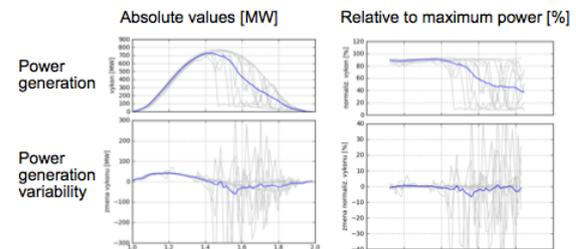
**Figure 7:** PV power generation and variability during sudden change of weather (daily profile in 30 May 2005). Blue profile: ČEPS TS, grey profiles: randomly selected 1 MWp PV power plants. Refer to the maps in Fig. 6.
