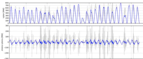
**Figure 5:** Daily PV power generation profiles (above) and the related variability (below) assuming complete portfolio of PV power at the level of the Transmission System (blue colour), and assuming 10 randomly selected 1 MWp PV plants in the country (grey colour).
